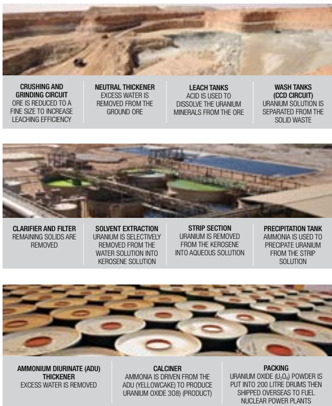
Figure 3: Steps in processing uranium ore
