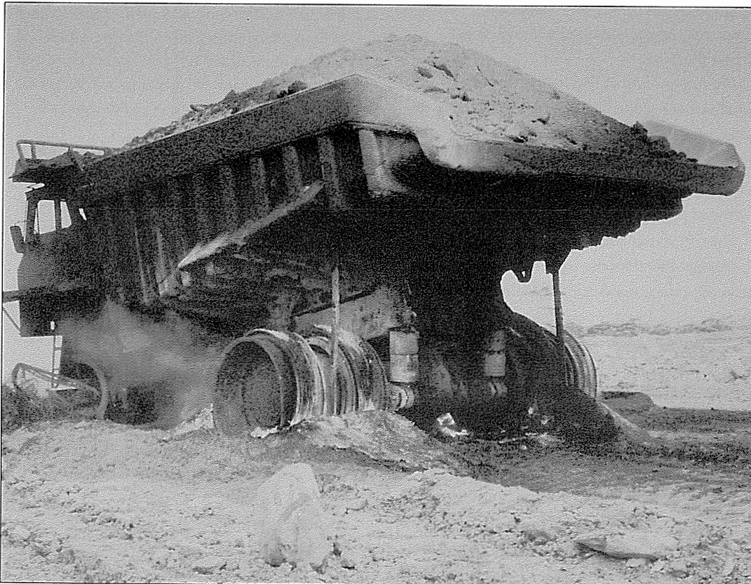
Accidents are a constant worry to the Department. Here, an expensive ore truck is wrecked by fire after making contact with an overhead power line at a mine site near Kalgoorlie.
