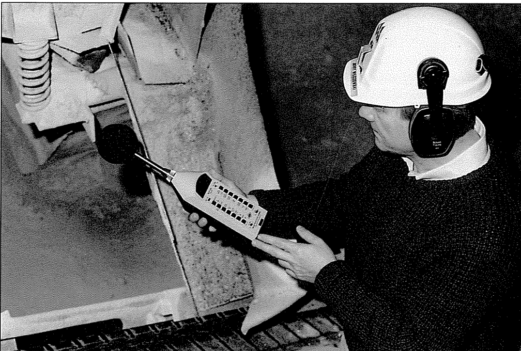
Special Inspector of Mines Jerry Wilczewski checking noise emission levels from a mining company's processing plant.
