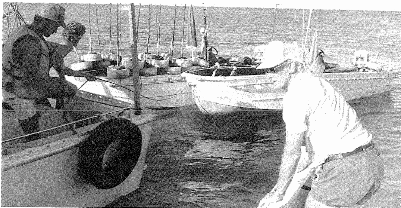
Using Teleseis for seismic surveying in shallow water. This technique uses floating transmitters to beam the data from individual seafloor geophones to a recorder vessel in deeper water or a station on adjoining land.
