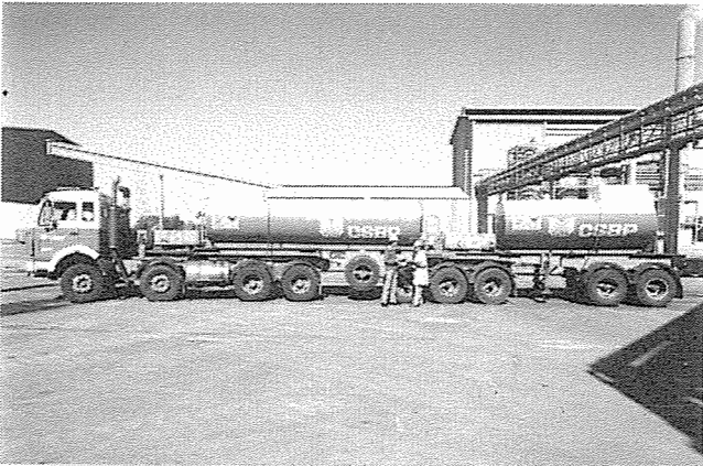
A typical B Train ready for loading with concentrated sulphuric acid. Emergency Information Panels are in place and the driver is wearing appropriate protective clothing.
