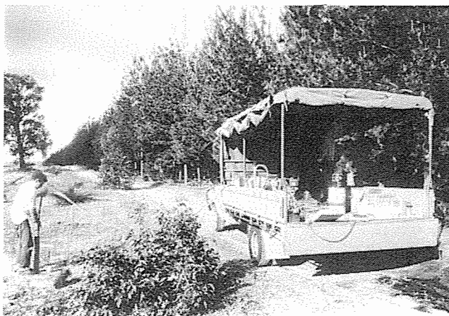
Lowering an air-driven pump into a shallow drillhole to obtain a pumped water sample.
