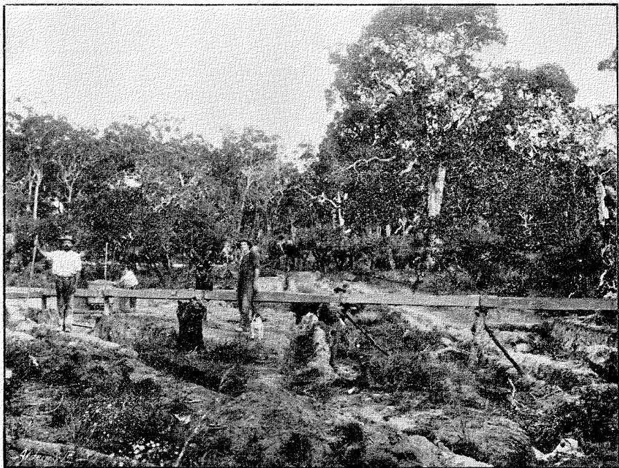
Ground Sluicing, Greenbushes.
